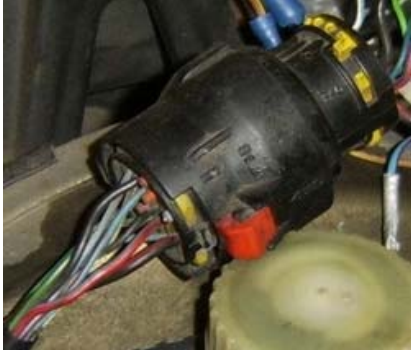
Stecker X5 – Calibra / Vectra A C20XE (Motorraum)
